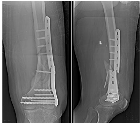
Fig 3: X ray of broken implant
